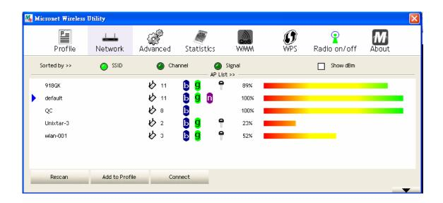
If the access point selected does not use encryption, it will connect to this device within one minute. If the access point selected uses encryption, please proceed to step 3.
